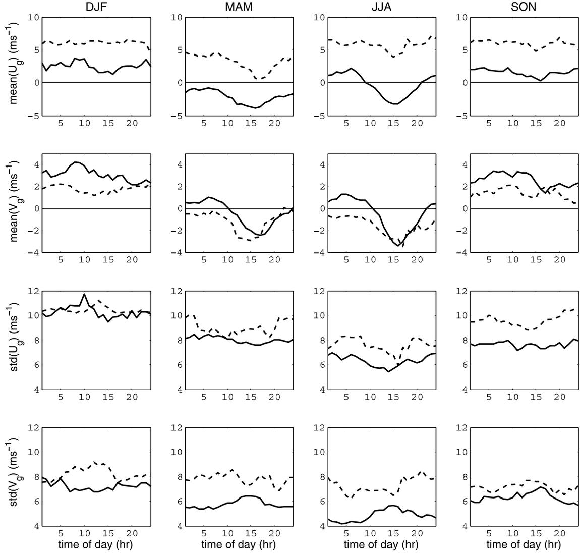
**Figure 3.** Diurnal variations of the mean and standard deviation of the surface geostrophic wind components  $U_g$  and  $V_g$  under clear-sky (solid) and LLC (dashed) conditions at the Cabauw site for all seasons from 2007 to 2011.
