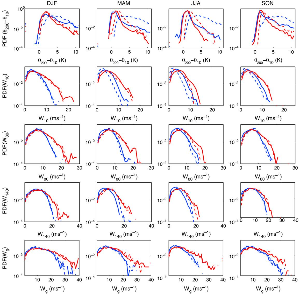
**Figure 2.** The pdf (logarithmically scaled) of potential temperature stratification between 200 m and 10 m ( $\theta_{200} - \theta_{10}$ ); wind speed at 10 m ( $W_{10}$ ), 80 m ( $W_{80}$ ), and 140 m ( $W_{140}$ ); and the surface geostrophic wind speed ( $W_g$ ) during daytime (7 A.M. to 7 P.M.) (solid) and nighttime (7 P.M. to 7 A.M.) (dashed) under clear sky (blue) and LLC (red) at the Cabauw site for each of the seasons from 2007 to 2011.
